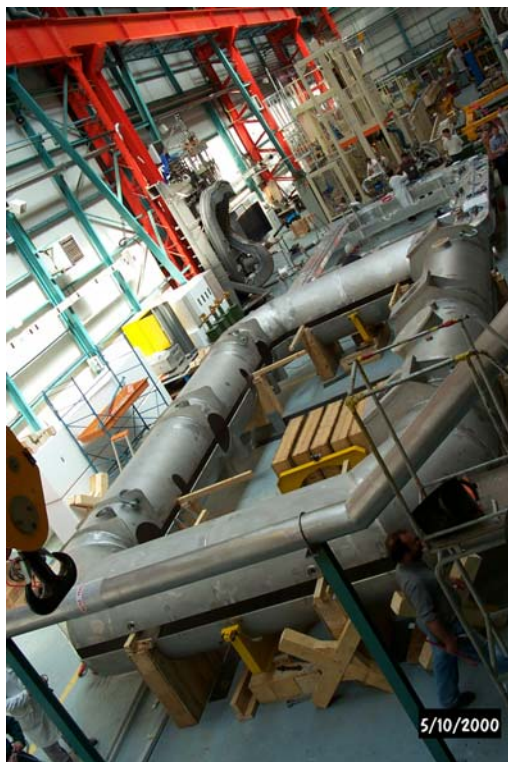
Fig. 3. Integration of the B0 cold mass in the vacuum vessel.
