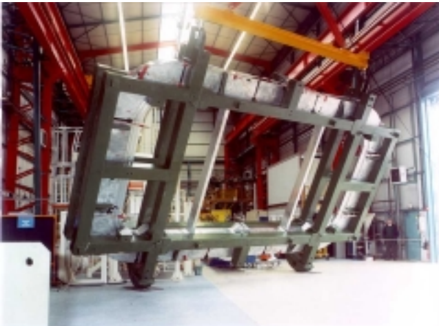
Fig 4 Handling of the B0 Coil cold mass
