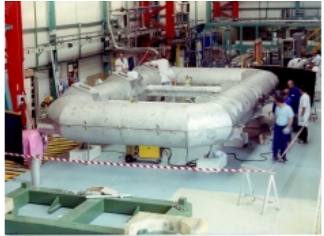
Fig. 9 The B0 vacuum vessel under final completion
